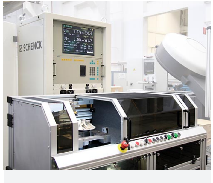
Various balancing units (up to 3) can be combined for fast balancing of a wide range of turbocharger rotors without requiring costly change over.
