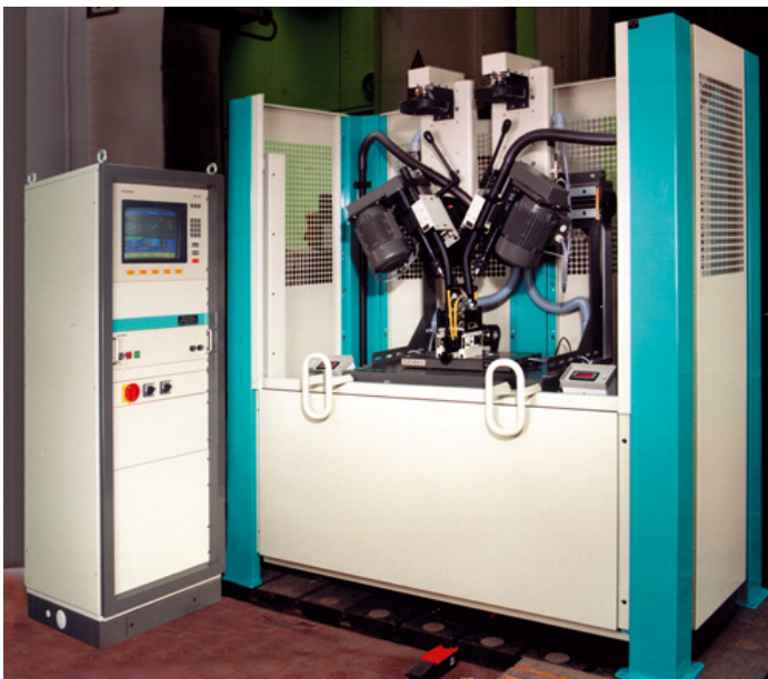
In this H10-BK balancing machine for rotors up to 16 kg, vertical correction units were adapted with swivelling drill units. Unbalance correction with radial and inclined drilling directions are no problem with this arrangement.
