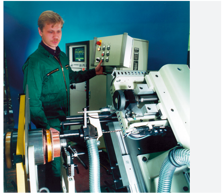
All modules are ergonomically designed with a view toward simple operation. Valuable time is saved by a motorized feed mechanism for the processing unit, the pneumatic spindle feed or the display unit for the required correction.
