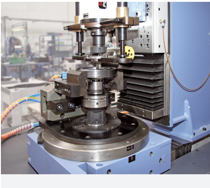
Fully automatic machine for balancing pulleys or vibration dampers, featuring manual loading and unloading. The numerically controlled milling unit can be changed over to a new workpiece type at the push of a button, and ensures highly precise unbalance correction.
