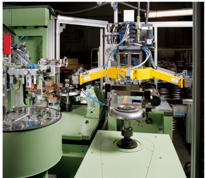
Multiple-station balancing machine with diagonally arranged welding system for unbalance correction on turbines. Correction is made with the help of fixed weights dispensed by a shaking system and supplied one-by-one to the welding electrode. The angle between the two weights is varied depending on the unbalance.
