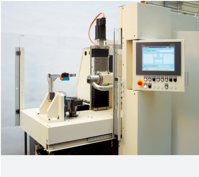
Horizontally arranged milling unit for radial unbalance correction on an articulated flange. If the unbalance cannot be removed in a single milling operation, correction is made in multiple components as required.
