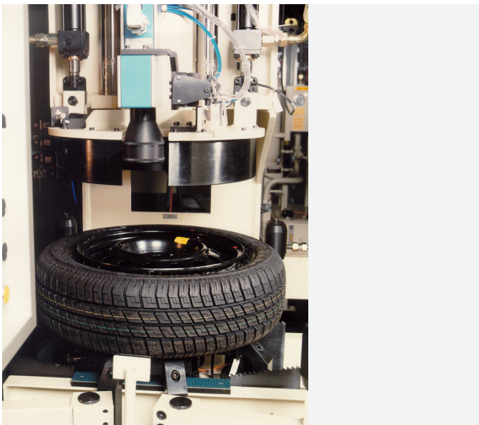
Optional matching station for improving the behavior of the wheel on the vehicle. The matching points on the un-inflated tire and rim are identified and brought together. The rim is radially clamped from the inside and the tire is gripped from above and below. The rim can then be rotated to achieve the optimum matching angle.
