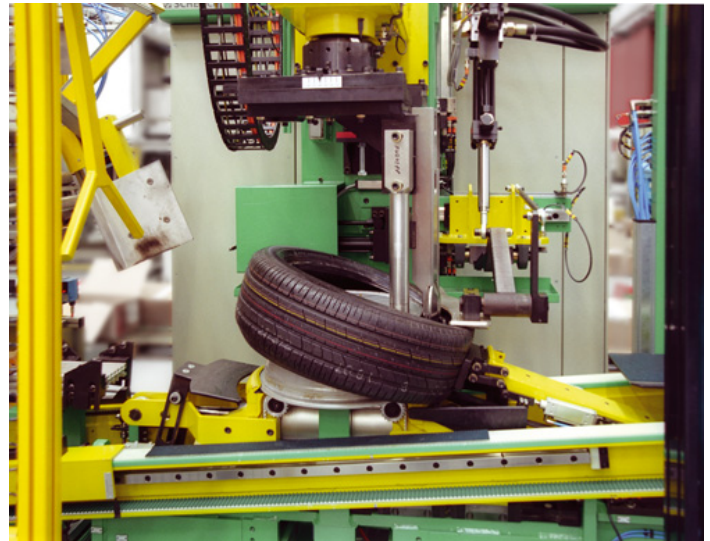
Mounting station with single-armed design of the mounting head for gentle mounting of the tire. Automatic lowering of the mounting head to the detected rim width with simultaneous, automatic adjustment to the detected rim diameter. When the mounting head lowers, the tire hold-down roller and tire-pusher are adjusted to optimally position the tire. With a width-height ratio less than 60% it is recommended that the two beads be mounted one at a time in two revolutions.
