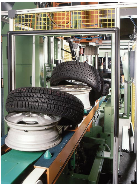
Automatic transport of the tire within the system through a turn-and-lift conveyor. The complete cycle then runs automatically. All the operator has to do is load lubricated tires and rims.
