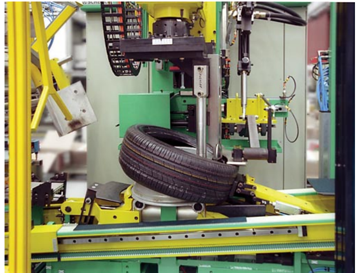
The tire mounting procedure takes only a few seconds. The heart of the system is the non-contacting draw-down head that prevents damage to the rim and especially the edge. Mounting of the two tire beads is selectively done either both at the same time, or one bead at a time in two revolutions. The machine can be changed over easily and in a short time and therefore a large tire-diameter range of steel and alloy rims can be handled. In the basic version the machine is installed between two feed conveyors and manually loaded. The rims and tires are manually supplied in sets according to the manufacturing orders. If a new type of tire is to be processed, only the draw-down head has to be adapted to the new rim diameter. Automatic change over is optional.
