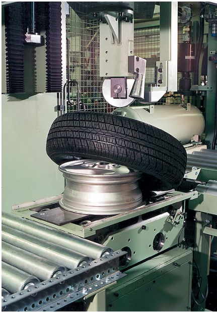
This assembly head provides diameter adjustment in steps. The change over to another rim diameter can be done manually by push-button or fully automatically by a type identification system.
