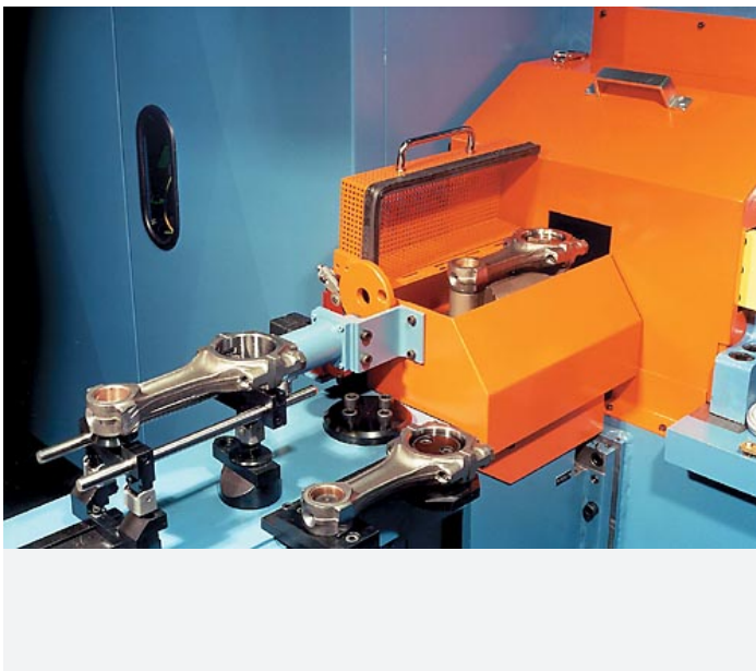
Measurement and check weighers each with two electronic load-cells for the big-end and small-end. Digital determination of absolute weight or deviation from pre-defined target weight. Zero setting according to a master connecting-rod. Weigher adaptable to other work-piece types by adjustment or exchange of the adapter.
