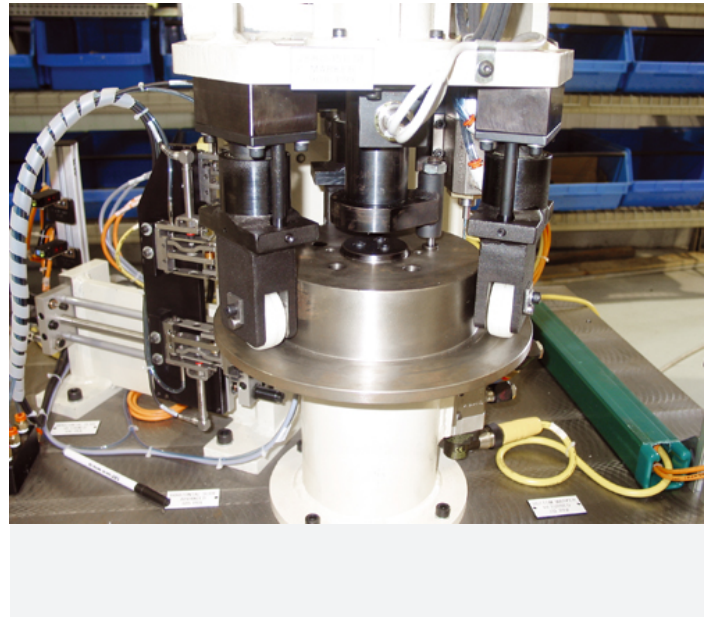
This system determines the characteristics of a brake disc. The machine works fully automatically and is loaded by means of a handling system. Characteristics measured include: Lateral and radial runout, Waviness, Diameter, FFT analysis, Inclusion of temperature coefficient.
