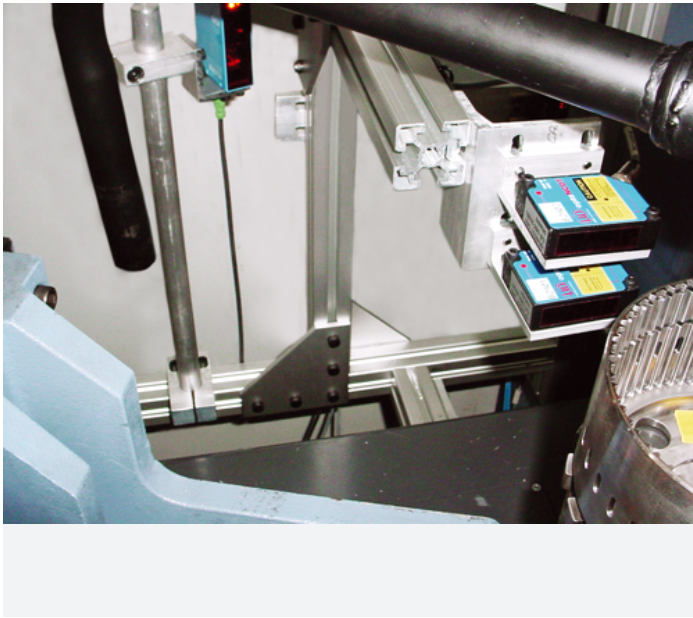
Runout measurement on gearbox components integrated in a fully automatic vertical balancing machine. Runout is measured during the unbalance measurement run. If unbalance and runout are within tolerance, the work-piece is deposited on the „Within Tolerance“ conveyor.
