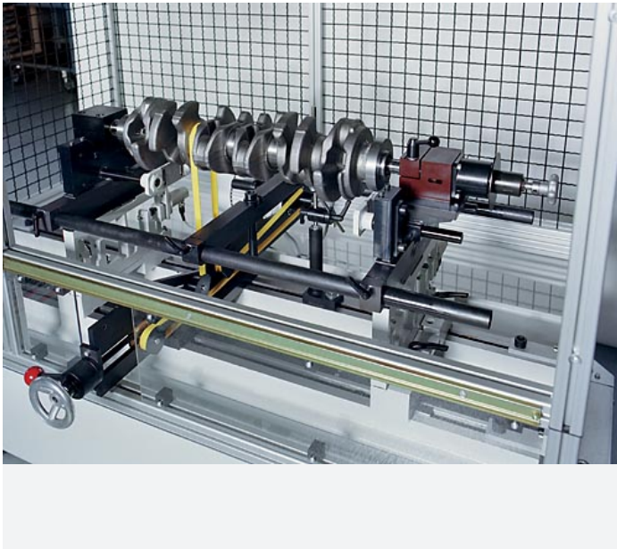
Crankshaft casting supported in rotating spindle cones. Suitable for symmetrical crankshafts. Equipped with belt-drive and angle reference through a single-mark on the rotor. Optional precision roller carriages for directmounting of finish-machined crankshafts.
