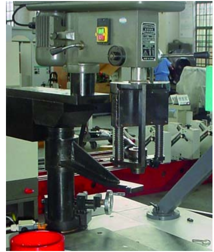
machine with integrated correction drilling unit
