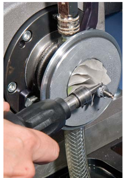
Correction with optional hand grinder
