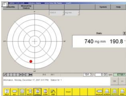
Vector indication of the unbalance
