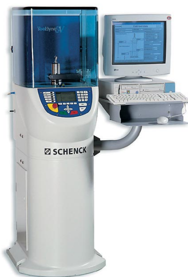
The vertical design of the machine with hard-bearing principle simplifies not only the operation, but also – through permanent calibration – the setup of the measuring equipment. A pneumatically activated, quick-acting clamping mechanism makes loading the machine easy and guarantees repeatable tool seating. An indexing aid with laser indicator assists in accurately locating the exact correction position.
