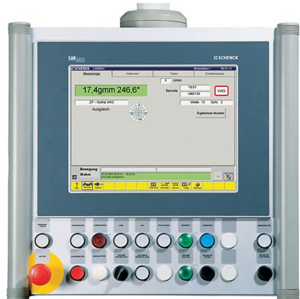
Ergonomic PC-based measuring unit with TFT touch screen display. Optimum calculation of unbalance correction masses to be removed by drilling, with direct display. Digital measuring process with high frequency selectivity. Compensation circuit for electrical compensation of initial unbalance or adapter unbalance. Further special features: Large display, operator prompting, diagnostic programs, fault display, statistics program and printer connection. Measuring unit prepared for remote diagnosis through interface.
