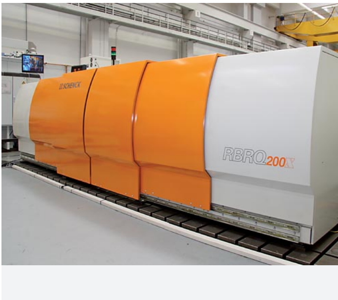
Standard protective safety guarding in modular elements with laminated plates for burst and noise protection. Quick acting pneumatic actuation of the large horizontally opening doors. Camera and monitor replace viewing windows.
