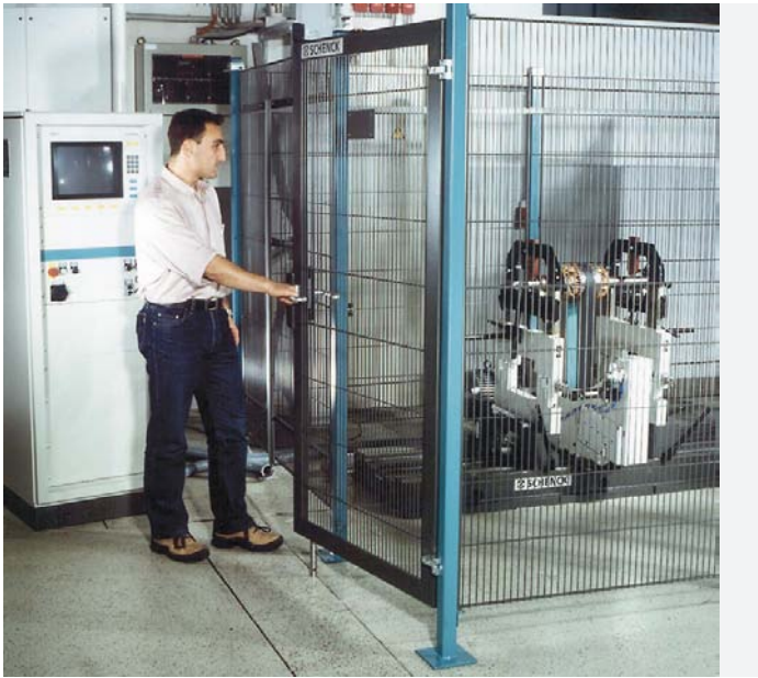
Very good access to the rotor and machine is achieved with a protection class B enclosure. The protective fence permits simple adaptation to every space requirement.
