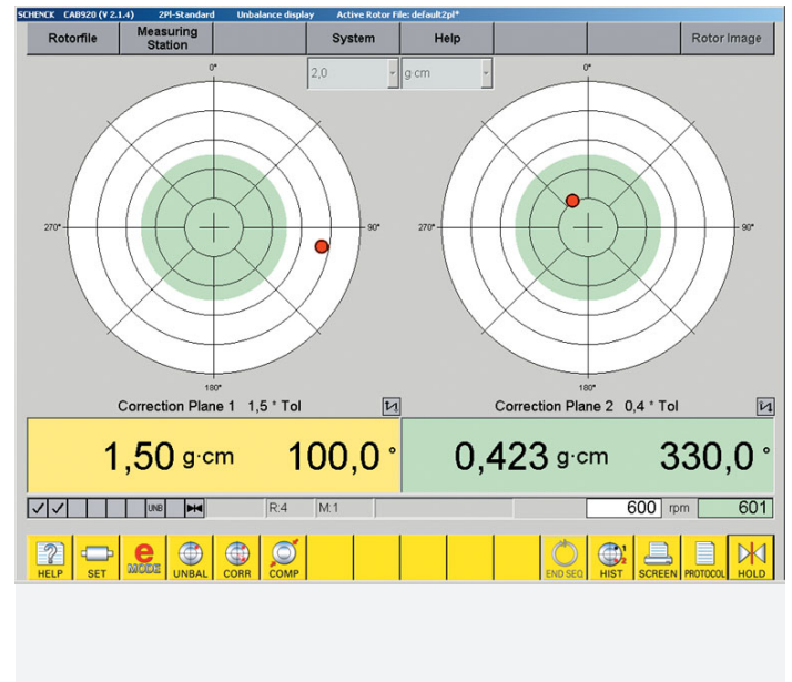
Clear vectorial and numerical display of the unbalance with coloured marking when the tolerance is reached
