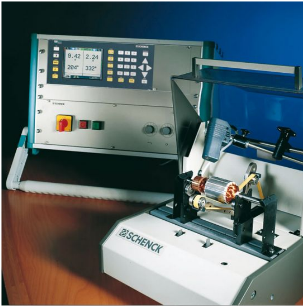
Balancing made simple with CAB 700, irrespective of whether the rotor is small or large.
