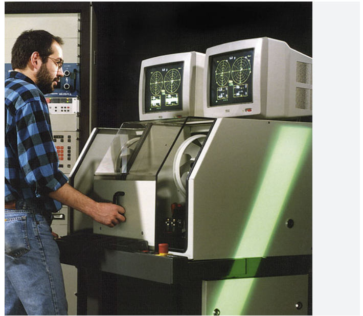
For larger batches, a two-station machine is the optimum solution. The machine can be operated in overlapping cycle, i.e. while the unbalance of one rotor is being corrected, the unbalance of the next one can already be measured. Likewise, the operating and safety concept is designed with a view to short cycle times.
