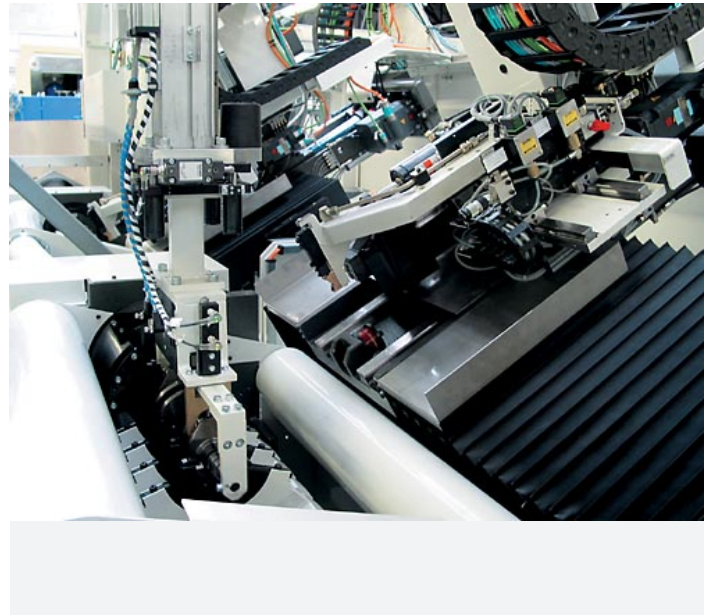
Correction stations with easy-access, horizontally-arranged drill unit with electro-mechanical feed mechanism. Precise touch point signal and depth-control. Drill with coolant or oil. Clamping unit completely enclosed, to prevent contamination of the machine by coolant and chips. Chip removal by under-floor chute or chip conveyor.
