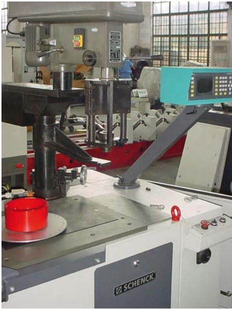
Drilling correction unit, including swarf extractor system (option)
