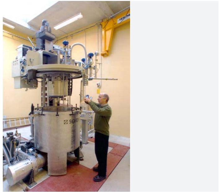
Cryogenic overspeed test stand for tests with temperatures close to absolute zero
